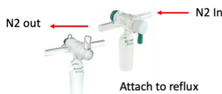
Fig 6: Adapter to bring in nitrogen (Chemglass AF-0509-B) .
